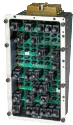
56 CB military helicopter panel (PCB + casing)
