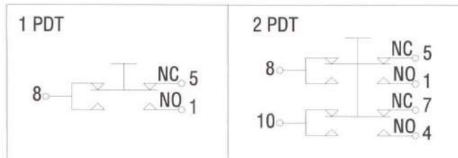
Form "C" Switch Circuits
