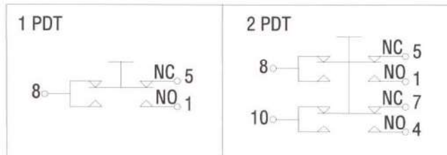
Form "C" Switch Circuits
