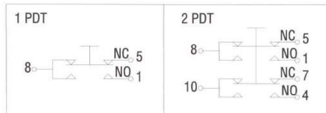
Form "C" Switch Circuits
