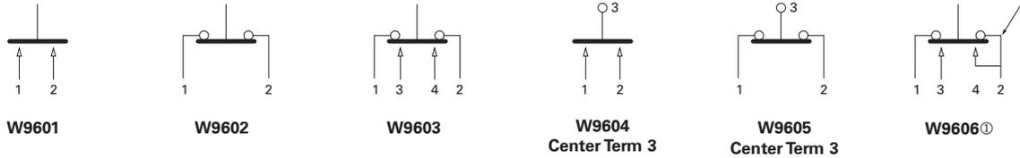
① For W9606 or SPDT circuit, mount terminal jumper to terminal #2 and #4.
