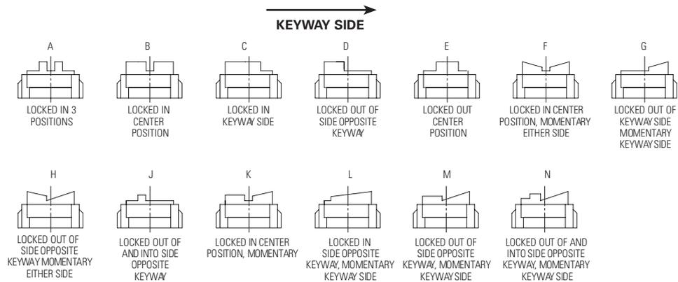
Figures A thru N do not represent details of construction. They schematically illustrate locking function.
