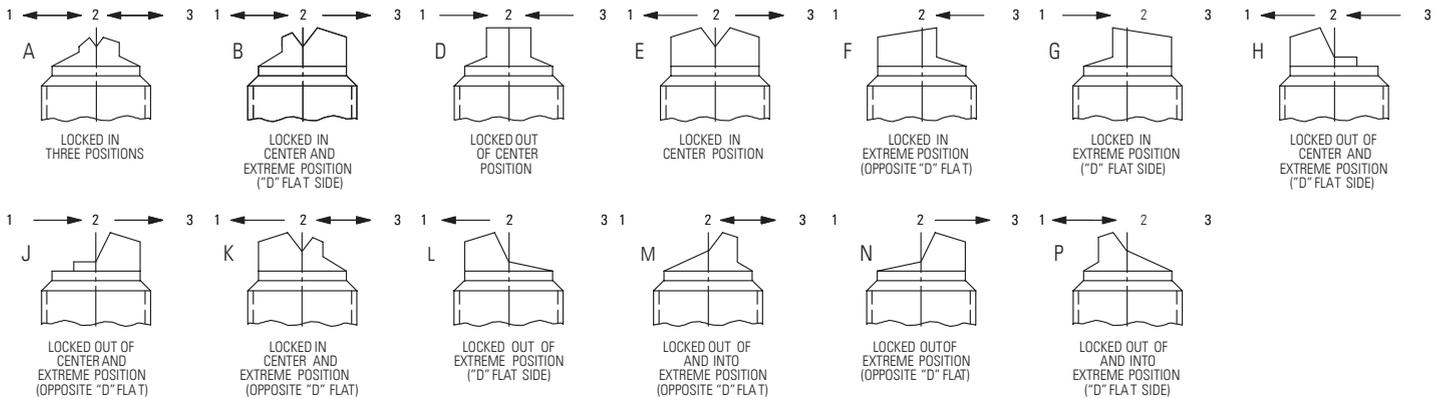
Notes: 1. Arrows (<>) indicated lever must be unlocked to move against the arrow direction.
