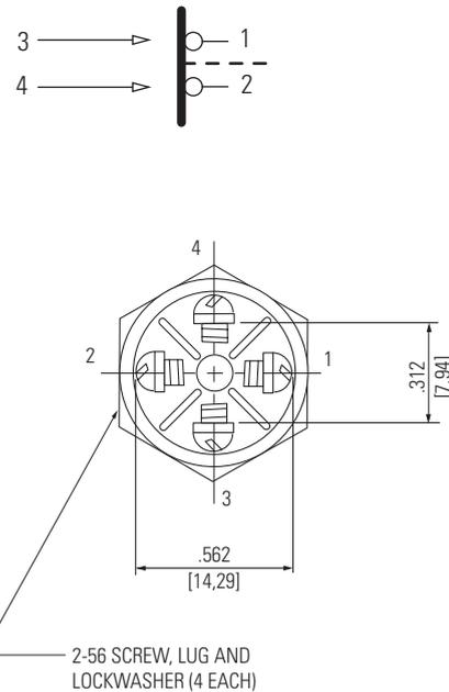
Mounting and terminal hardware supplied unassembled.
