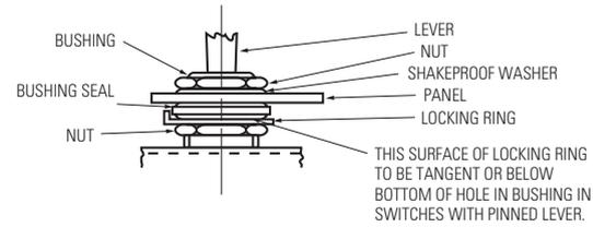
BUSHING SEAL TO BE ASSEMBLED SO THAT SURFACE, WITH MARKING "BOTTOM," IS DOWN. LOCKING RING CAN BE ASSEMBLED WITH EAR EITHER UP OR DOWN.
